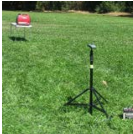
Figure 1. Generator and sound level meter.
