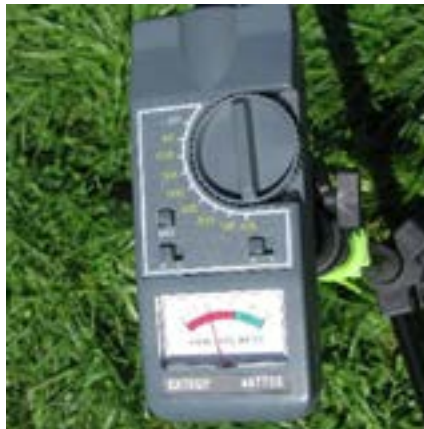
Figure 2. Analog sound level meter showing 60 dB(A).
